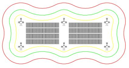
Dynamic determination of lightning protection areas is available in the latest versions of AutoCAD, BricsCAD, GstarCAD and ZWCAD.
