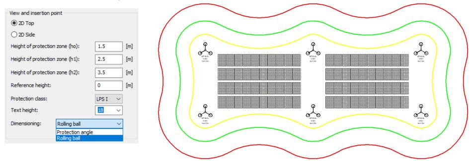
Dynamic determination of lightning protection areas is available in the latest versions of AutoCAD, BricsCAD, GstarCAD and ZWCAD.
